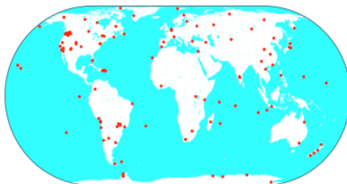
Figure 3 (below). The GDGPS network which provides global real-time GPS coverage for research and applications. GDGPS provides streams of positions for all sites at 1 sample per second. Figure from http://www.gdgps.net/ courtesy of Yoaz Bar-Sever.
